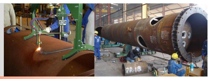
The KHC-600D is ideally suited for cutting high precision T- joint circles including any hole that crosses the side of the pipe for piping systems, high pressure vessels and heat exchangers. Developed with KOIKE Advanced Technology, the KHC-600D is a compact design that is light weight and easy to operate. In addition to cutting circles and bevel in flat plate, the machine can cut holes in vessels from the inside or outside.
