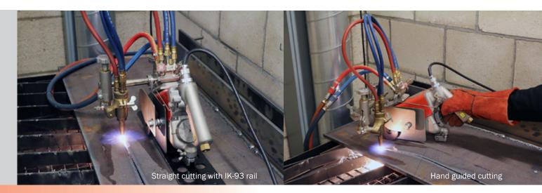
The IK-93T Hawk is a portable gas cutting machine developed primarily for the purpose of high quality straight line, hand guided cutting. In addition to featuring high cutting quality, it also demonstrates unprecedented smooth operation and mobility.
