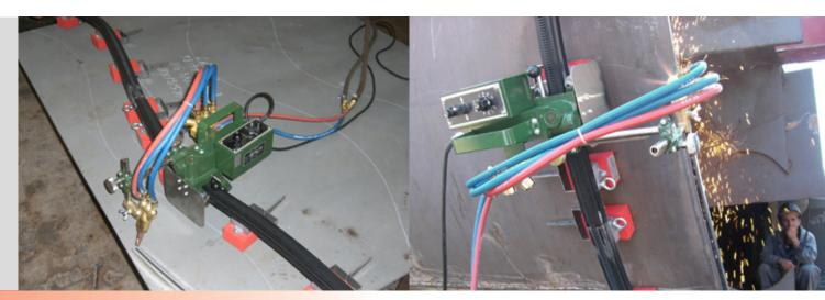
The IK-72T cuts various types of steel shapes including channel, curved plate and angled steel members. Made of an aluminium alloy, the IK-72T is lightweight and easy to handle. A graduated bevel collar is provided for bevelling. Simply adjust the scale to precise bevel angle.
