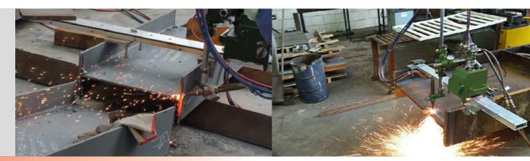
The Mini-Mantis II is a semi-automatic gas cutting unit for rapid and precise cutting of H-beams. The rotatable torch angle allows bevelling cuts on flange and web. The vertical unit can be tiles for cutting flanges in angled directions. KOIKE's quality construction ensures durability and trouble-free operation. The Mini-Mantis II is an economical, efficient and compact gas cutting machine for H-beam steel.
