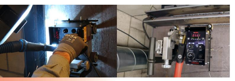
The Wel-Handy Mini Strong is a compact design welding carriage designed to perform horizontal, vertical, and overhang welding. A 35 kg magnet and 16 kg traction power provides reliable performance and quality welds. The machine is easily carried around with the handle with magnet detachment mechanism.
