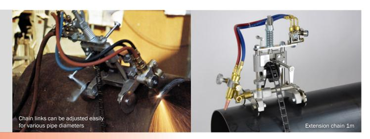
The Picle-1 is a manually operated pipe cutting machine for cutting and bevelling pipes. Equipped with a chain and worm gear drive system with low transmission ratio, leading to an absolutely frictionless feel.
