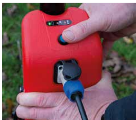
Floodlight operated from ground level switch
