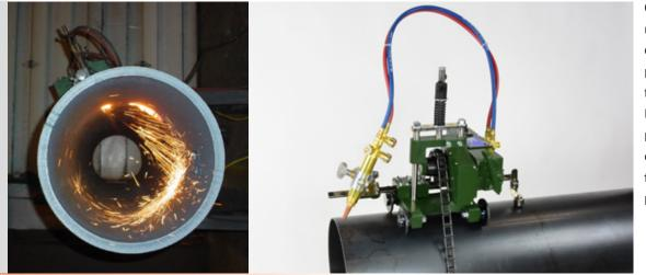
Optional guide rail provides high cutting accuracy, particularly suitable for large pipes. Each guide rail is provides with additional chain links for each maximum pipe diameter.
